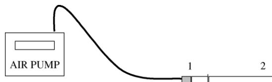
Fig. 1. Schematic diagram of the volatilization chamber: 1-C 18 cartridge and 2-PVC tube. For other details, see text.
